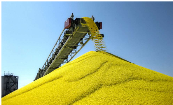
Figure 1. Wet prilled sulfur being conveyed from a sulfur prilling unit to a pile for open storage.
