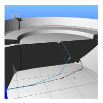
By design, our hard pipe system provides constant positive drainage and eliminates the risk of failure due to frozen product, often associated with alternative hose drains. Additionally, because our system is never in contact with the tank bottom, there is no potential for damage to the tanks coating due to friction.
